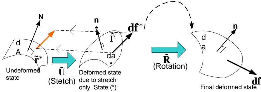
Biot-Lure  $\tilde{\mathbf{r}}^*$  Stress tensor exist in the undeformed state only
