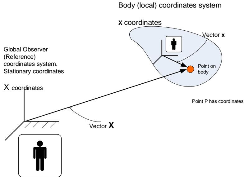
In general, the interest is in finding differential changes that occur when a body deformed. This mean measuring how a differential vector that represents the orientation of one point relative to another changes as a body deformed.
