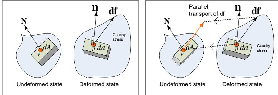
Step 1. Determine Cauchy stress in deformed state
