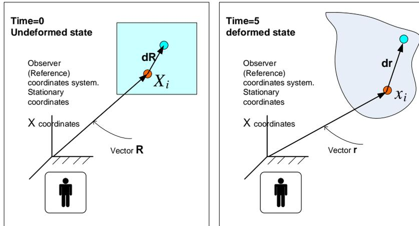
Another way to represent the above is by using the same diagram to show both the undeformed and the deformed configuration as follows.
