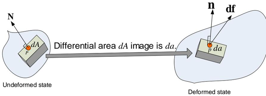
Differential area deformation and normal unit vectors used in stress measurement
