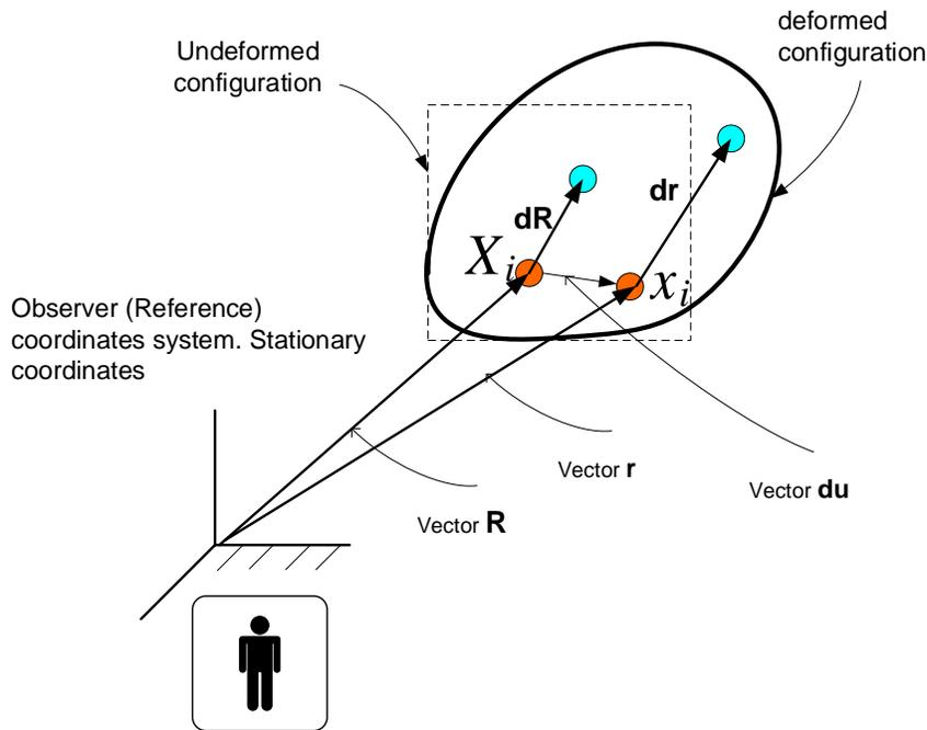
Let  $B$  be the undeformed configuration, referred to as the body *state*. By state it is meant the set of independent variables needed to fully describe the forces and geometry of the body.
