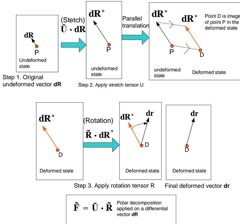
The effect of applying the deformation gradient tensor  $\tilde{\mathbf{F}}$  on a vector  $d\mathbf{R}$  can be considered to have the same result as the effect of first applying a stretch deforming tensor  $\tilde{\mathbf{U}}$  (Also called the deformation tensor) on  $d\mathbf{R}$ , resulting in a vector  $d\mathbf{R}^*$ , followed by applying a rotation deforming tensor  $\tilde{\mathbf{R}}$  on this new vector  $d\mathbf{R}^*$  to produce the final vector  $d\mathbf{r}$ .
