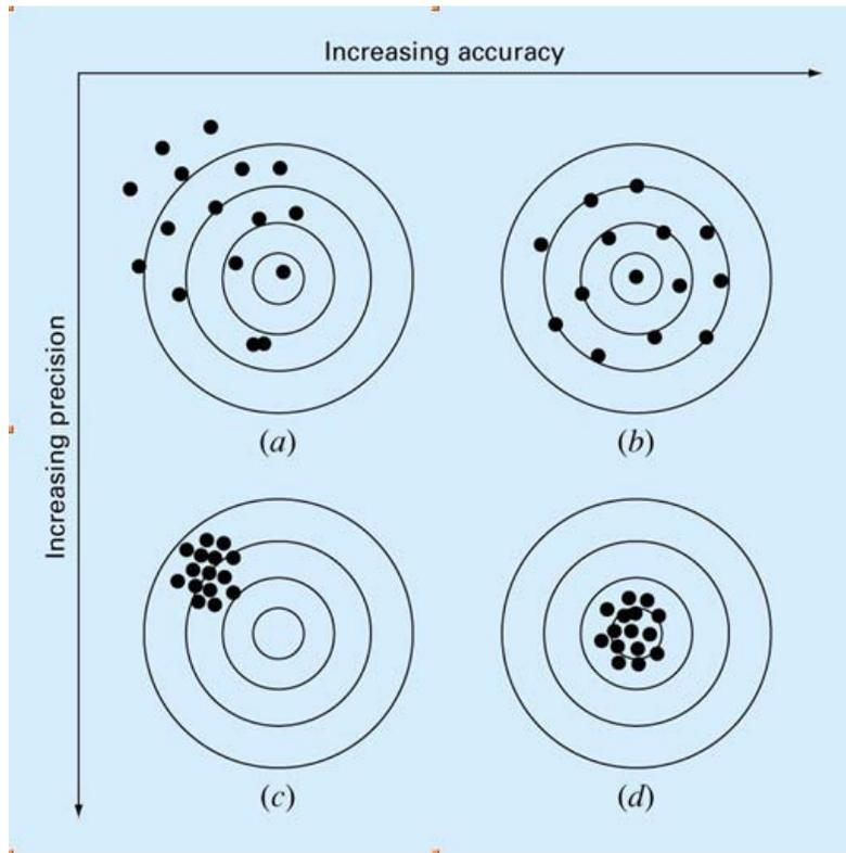
From the above dart diagram, then we can say this: a value is accurate if it is near the bull-eye. But if it is away from the bull-eye, but it is always away from the bull-eye and in the same place, then it is precise. So something can be precise but not accurate. So precision has to do with repeated values. i.e. one can't say a value is precise, but must talk about an experiment being precise, it is produced same result each time (or very close results each time).
