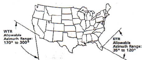
Fig. 4.3 Acceptable launch azimuth range for the United States.
