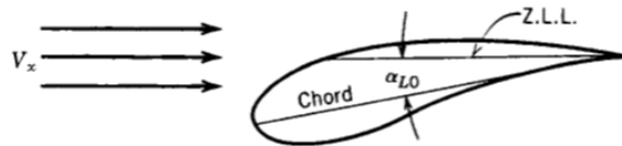
Fig. 5.11. Orientation of airfoil at zero lift.
