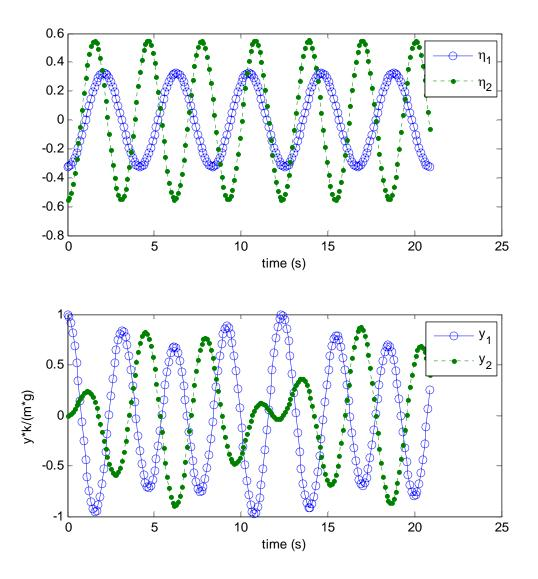
Response plotted over 5 cycles. Notice that the initial conditions are satisfied. Both modes are excited and oscillate at different frequencies. The superposition of both modes causes the response in y1, y2 coordinates to look quite complicated.
