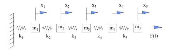
In parallel with each of the springs  $k_i$  which are drawn, there are viscous dampers  $c_i$  which are not shown. The equations of motion for this system are easily found to be:
