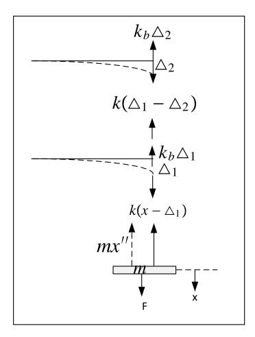
Applying equilibrium of vertical forces  $\sum F_v = 0$  for mass *m* and noting that inertial forces opposes motion, results in the equation of motion
