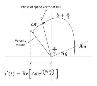
The difference is that the velocity vector has phase of  $\theta + \frac{\pi}{2}$  instead of  $\theta$  as was the case with the position vector, and the amplitude is  $A\omega$  instead of A. Hence the first time the
