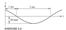
Use the properties in this trace to determine (a) The initial values of x and  $\dot{x}$ .
