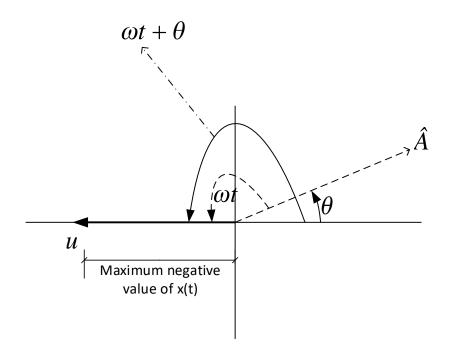
The minimum x(t) (in negative sense and not in absolute value sense) occurs when  $\omega t_{min} + \theta = \pi$ , hence  $t_{min} = \frac{\pi - \theta}{\omega}$ , therefore  $t_{min} = 2.5$
