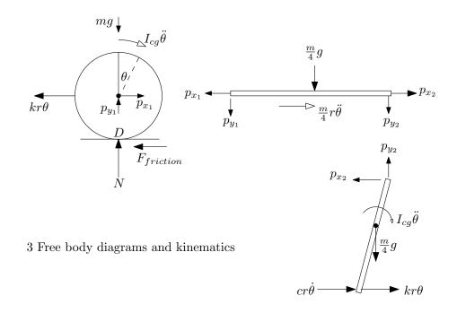
In this diagram, it is assumed the horizontal bar only moves in the x direction and this is all for small angle  $\theta$ . Now we apply Newton laws to each body.
