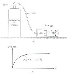
Solve for the complete response of the piston by using direct integration.
