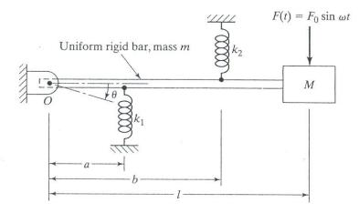
The free body diagram and the inertial diagram are given below. It is assumed that motion is measured from equilibrium position with the mass already in attached to springs. Hence the weight of the beam do not show up in the FBD.
