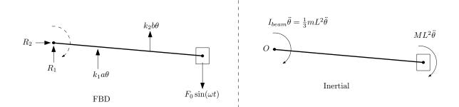
Taking moments around hinge at point o and using anti-clockwise as positive gives (assuming small angle  $\theta$ )
