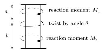
From mechanics of materials, there is relation between the twisting angle and resisting torque by beam which is given by
