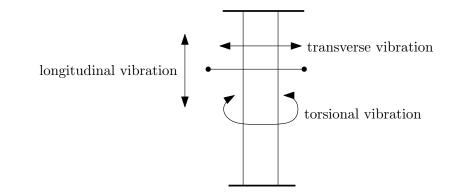
longitudinal In this mode the system can be modeled as the following
