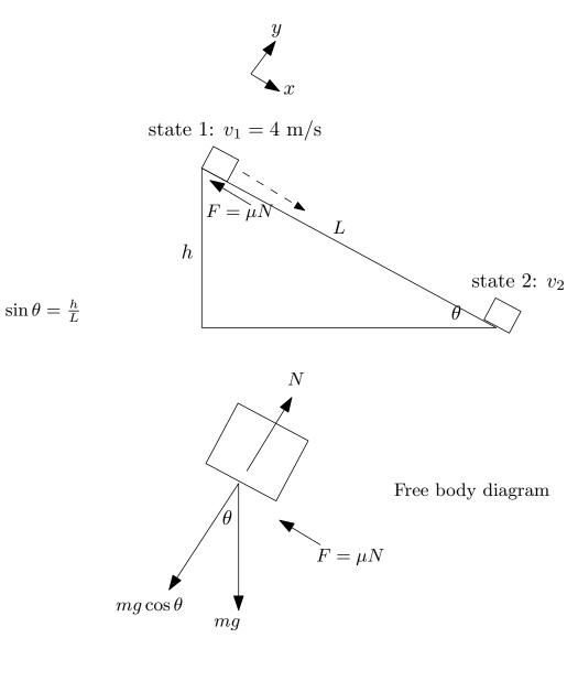
Work-energy is used. There are two states. First state is at the top and the second state is when child reaches the bottom of the hill. Zero datum for gravity potential energy is taken at the bottom of the hill.
