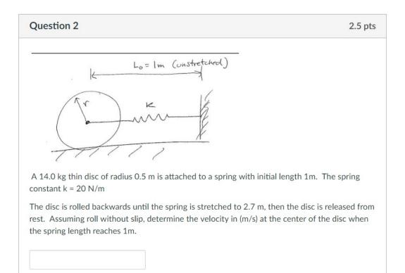
When the disk is pulled, it gains potential energy  $V_1 = \frac{1}{2}kx^2$  where x is amount of spring extension from equilibrium, which is 1.7 meter in this example. When released, all this energy will be converted to kinetic energy when the disk reaches its original equilibrium position. The final kinetic energy is  $T_2 = \frac{1}{2}mv_g^2 + \frac{1}{2}I_{cg}\omega^2$ . But since the disk rolls without slip, then  $v_{cg} = r\omega$  and
