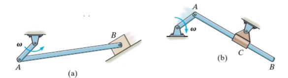
**1C** (**6 points**) For a given instant, a rigid body has velocity at point A parallel to the velocity at point B. Does this guarantee that the angular velocity of body is zero at this instant?
