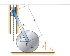
The system shown consists of a wheel of radius R = 12 in. rolling on a horizontal surface. A bar *AB* of length L = 35 in. is pin-connected to the center of the wheel and to a slider *A* that is constrained to move along a vertical guide. Poin*C* is the bar's midpoint. If, when  $\theta = 77^{\circ}$ , the wheel is moving to the right so that  $v_B = 5$  ft/s, determine the angular velocity of the bar as well as the velocity of the slider A.
