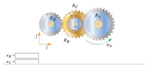
The tangential acceleration at the point where disk *A* and disk *B* meet is  $R_A \alpha_A$ . But this is also must be the same as  $R_B \alpha_B$  since the gears assumed not to slip against each others. Therefore
