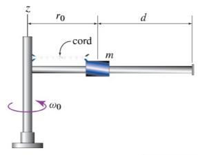
The collar will impact the end of the arm with a speed of m/s.
