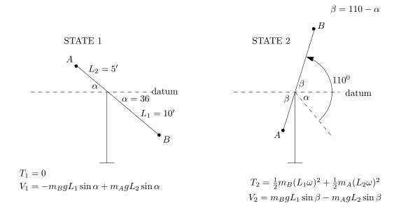
$T_1 + V_1 + U_{12}^{internal} + U_{12}^{external} = T_2 + V_2$ But  $U_{12} = 0$  since there is no friction and no external forces. Now  $T_1 = 0$  since at rest. And  $V_1 = -m_B g L_1 \sin \alpha + m_A g L_2 \sin \alpha$
