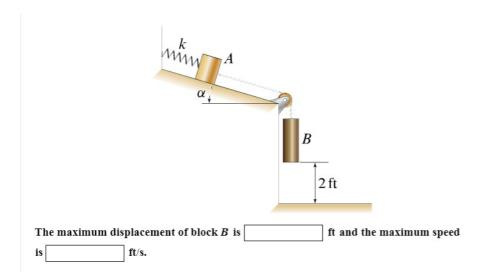
maximum displacement is 2 ft. Maximum speed is 9.404 ft/sec.
