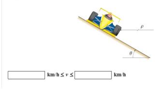
For maximum speed, friction acts downwards as car assumed to be just about to slide upwards. Resolving forces in normal and tangential gives
