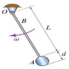
A pendulum consists of a uniform disk A of diameter d=0.16 m and mass  $m_A=0.37$  kg attached at the end of a uniform baB of length L=0.75 m and mass  $m_B=0.7$  kg. At the instant shown, the pendulum is swinging with an angular velocity  $\omega=0.23$  rad/s clockwise. Determine the kinetic energy of the pendulum at this instant, using  $\omega=0.23$  rad/s clockwise.
