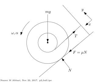
Notice that the Friction force F is pointing downwards since the spool is spinning counter clockwise. Resolving forces along x gives
