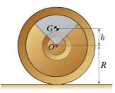
An eccentric wheel with weight W=260 lb, mass center G, and radius of gyration  $k_G=1.32$  ft is initially at rest in the position shown. Letting R=1.76 ft and h=0.6 ft, and assuming that the wheel is gently nudged to the right and rolls without slip, determine the speed of O when G is closest to the ground.
