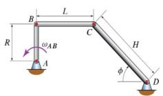
The weights of the uniform thin pin-connected bars AB, BC, and CD are  $W_{AB}=3$  lb,  $W_{BC}=6.5$  lb, and  $W_{CD}=11$  lb, respectively. Letting  $\varphi=49^\circ$ , R=4 ft, L=5.5 ft, and H=6.5 ft, and knowing that bar AB rotates at an angular velocity  $\omega_{AB}=3$  rad/s, compute the kinetic energyT of the system at the instant shown.  $T=\sqrt{100}$
