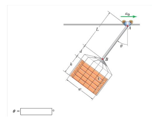
Let us assume the center of mass of the overall system is at some distance z from point A somewhere between A and C. It does not matter where it is. Therefore the rotational equation of motion for the hanging system is
