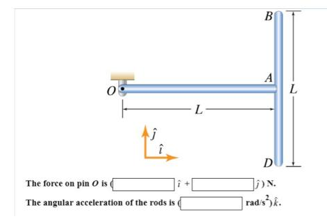
Resolving forces in x direction, where  $F_x, F_y$  are forces in hinge
