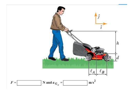
Taking moments about G (and assuming no friction from the ground as problems says to neglect rotational inertia of wheels, which seems to imply this).
