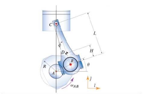
For the slider–crank mechanism shown, let R = 2.3 in., L = 5.3 in., and H = 1.5 in. Also, at the instant shown, let $\theta = 26^{\circ}$  and  $\omega_{AB} = 4,890$  rpm.
