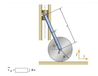
Since the wheel rolls without slip with angular velocity  $\omega_{disk} = 15$  rad/sec and its radius is  $r = \frac{5}{12}$  ft, then the center of the wheel moves to the left (since disk is rolling with counter clock wise) with velocity
