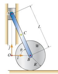
The system shown consists of a wheel of radius R = 1.58 m rolling without slip on a horizontal surface. A bar, AB, of length L = 3.43 m is pin-connected to the center of the wheel and to a slider, A, constrained to move along a vertical guide. Point C is the bar's midpoint.
