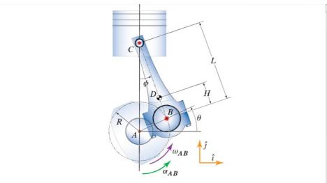
For the slider–crank mechanism shown above, let R = 2.1 in., L = 5.8 in., and H = 1.3 in. Assuming that  $\omega_{AB} = 5,030$  rpm and is constant, determine the angular acceleration of the
