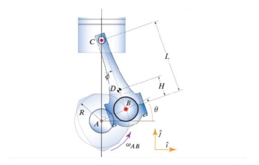
For the slider-crank mechanism shown, let R = 2.3 in., L = 5.3 in., and H = 1.5 in. Also, at the instant shown, let  $\theta = 26^{\circ}$  and  $\omega_{AB} = 4,890$  rpm. Determine the velocity of the piston at the instant shown.  $v_{C} = \boxed{\hat{j} ft/s}$
