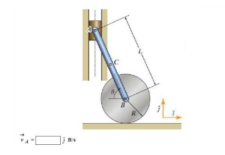
Since the wheel rolls without slip with angular velocity  $\omega_{disk} = 15$  rad/sec and its radius is  $r = \frac{5}{12}$  ft, then the center of the wheel moves to the left (since disk is rolling with counter
