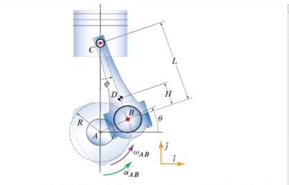
For the slider–crank mechanism shown above, let R = 2.1 in., L = 5.8 in., and H = 1.3 in. Assuming that  $\omega_{AB} = 5,030$  rpm and is constant, determine the angular acceleration of the
