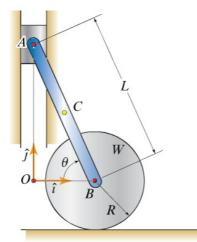
The system shown consists of a wheel of radius R = 1.58 m rolling without slip on a horizontal surface. A bar, 4B, of length L = 3.43 m is pin-connected to the center of the wheel and to a slider, 4, constrained to move along a vertical guide. Point C is the bar's midpoint.
