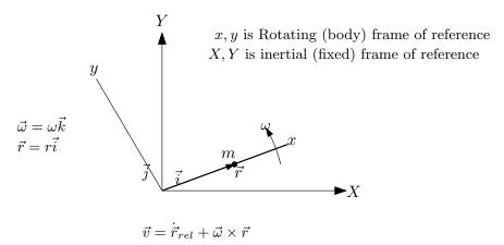
The position vector of the particle is  $\mathbf{r} = \mathbf{i}r$  where  $\mathbf{i}$  is unit vector along the x axis. Taking time derivative, and using the rotating vector time derivative rule which says that  $\frac{d\mathbf{A}}{dt} = \left(\frac{d\mathbf{A}}{dt}\right)_{relative} + \boldsymbol{\omega} \times \mathbf{A}$  where  $\boldsymbol{\omega}$  is the angular velocity of the rotating frame then
