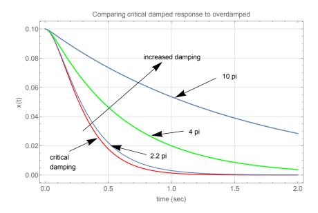
From the above we see that critical damping has the fastest decay of the response x(t). As the damping increases, it takes longer for the response to decay.
