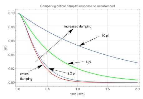
From the above we see that critical damping has the fastest decay of the response x(t). As the damping increases, it takes longer for the response to decay.
