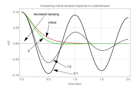
As the damping becomes smaller, more oscillation occur. The case for  $\lambda = 5s^{-1}$  had the smallest oscillation.
