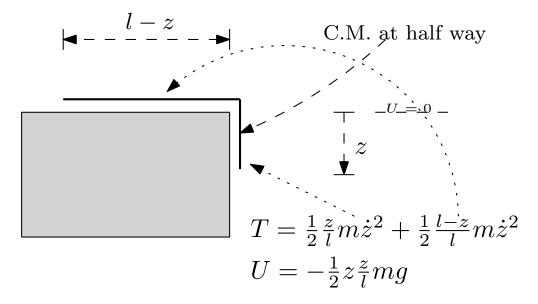
The top portion of the rope moves with same speed as the hanging portion. Hence z is used to describe the motion as the generalized coordinate. From the above
