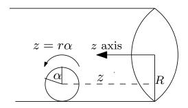
The sphere is now distance z away from the origin. There is new constraint now as shown
