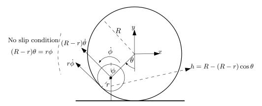
2 generalized coordinates  $\theta, \phi$  but constraint reduces this to one coordinate  $\theta$
