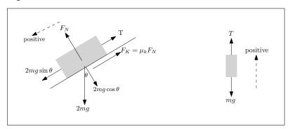
The acceleration of each body is the same. Let this acceleration be a. From the above free body diagram of the 2m body the equation of motion is now derived (using positive direction as show)
