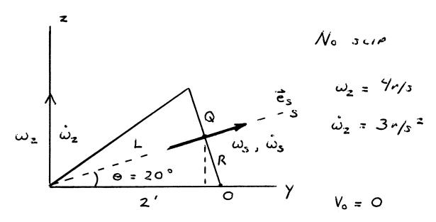
WS = SPIN ANGULAR UPLOCITY BUE TO NO SLIP CONDITION
