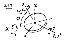
Given:  $\omega_z = 6000 \left(\frac{27}{60}\right)$  rad/s,  $\tilde{\omega}_z = 0$ , when  $\theta = 120^{\circ}$ :  $\dot{\theta} = 6$  rad/s,  $\ddot{\theta} = -90$  rad/s,  $\omega_z = 10$  rad/s,  $\dot{\omega}_z = 100$  rad/s. Find  $\tilde{\omega}_z \notin \mathbb{Z}$  at this instant. Solution: Fix xyz to the flywheel,
