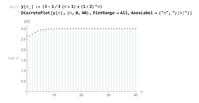
Figure 5: Plot of reponse y[n] to step input
