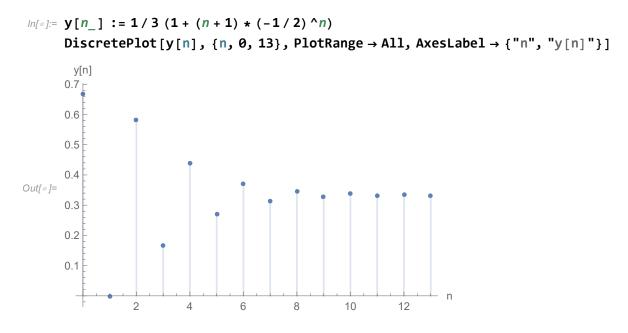
Figure 4: Plot of reponse y[n] to step input
