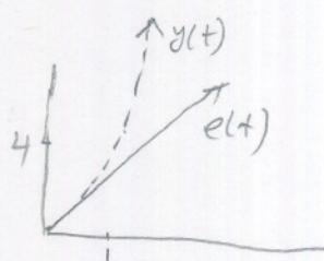
P+D  $\frac{Y(s)}{E(s)} = K_p \left(1 + T_d s\right) \Rightarrow Y(s) = (K_p + K_p T_d s) \frac{1}{s^2} \Rightarrow Y(s) = \frac{4}{s^2} + \frac{3.2}{s}$
