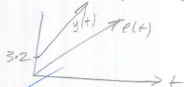
PID  $\frac{Y(s)}{E(s)} = K_p \left(1 + \frac{1}{T_i s} + T_d s\right) \Rightarrow Y(s) = \left(4 + \frac{4}{2s} + (4)(0.8)s\right) \frac{1}{s^2}$
