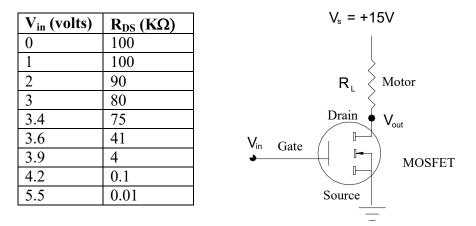
a) To make the motor spin, should the input gate voltage (V<sub>in</sub>) to the MOSFET be high or low and why?
