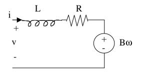
where  $\omega$  is the angular velocity of the motor shaft.
