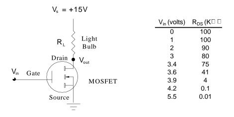
a) To turn the light bulb on, should the input gate voltage ( $V_{in}$ ) to the MOSFET be high or low?
