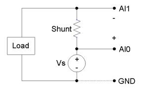
Figure 2-3. Differential measurement.
