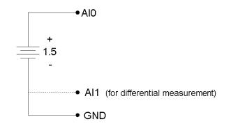
Figure 2-2. Single-ended measurement.
