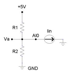
Figure 2-4. Single-ended measurement with voltage divider circuit.
