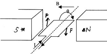
b. For the rest of this problem, assume the commutation is working. Draw the circuit model, and write the circuit equation describing the motor:
