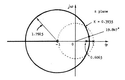
The value of gain K that will yield the damping ratio 5 of the closed-loop poles equal to 0.5 can be determined from Eqs. (4-53) and (4-54). Since T is given as 0.1 sec, we have
