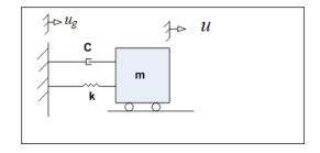
Where in the above, u is the absolute displacement of the tower, and  $u_g$  is the absolute displacement of the ground. The free body diagram is
