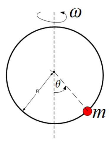
Kinetic energy T is made up of 2 components, one due to motion of the bead along the hoop itself with speed  $R\dot{\theta}$ , and another due to motion with angular speed  $\omega$  which has speed given by  $R\sin\theta\omega$  Hence
