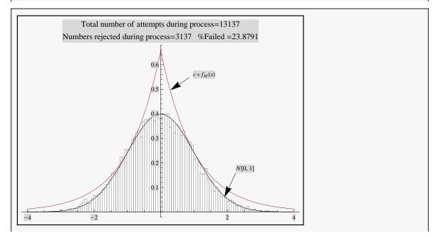
The above is a plot showing the histogram for random numbers generated using the accept - reject method for N=10,000. The random numbers are very close the N[0,1] which indicates this method is working well. The larger N is, the more closely the random numbers histogram will approach N[0,1] probability density.
