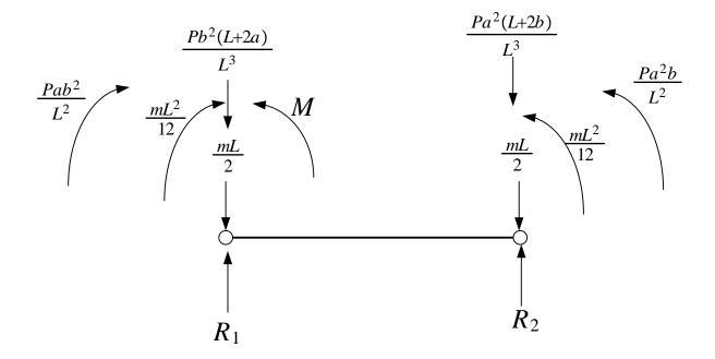
Now that all loads are on the nodes, the stiffness equation is applied
