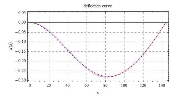
In the above, the blue dashed curve is the analytical solution, and the red curve is the finite elements solution using 2 elements. It can be seen that the finite element solution for the deflection is now in a very good agreement with the analytical solution.
