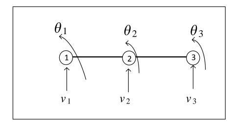
The stiffness matrix for each element is found and then the global stiffness matrix is assembled. Then  $\{p_{global}\}=[K_{global}]\{d_{global}\}$  is solved as before. The first step is to move all loads to the nodes as was done before. This is done for each element. The formulas for equivalent loads remain the same, but now L becomes L/2. The following diagram show the equivalent loading for P
