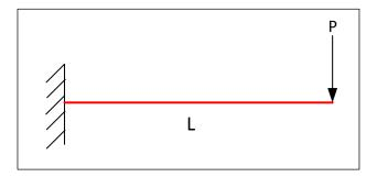
The first step is to make the free body diagram and show all moments and forces at the nodes
