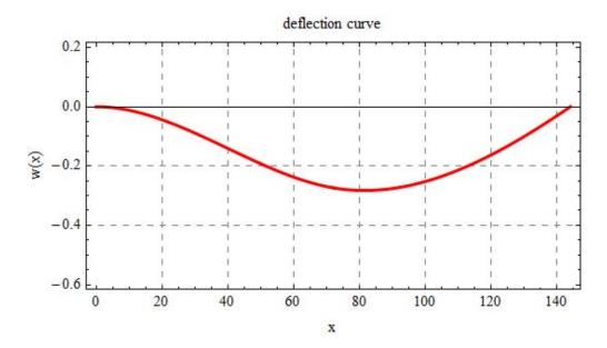
When the above plot is compared to the case with one element, the deflection is seen to be larger now. Comparing the above to the analytical solution shows that the deflection now is almost exactly the same as the analytical solution. Hence by using only two elements instead of one element, the solution has become more accurate and almost agrees with the analytical solution.
