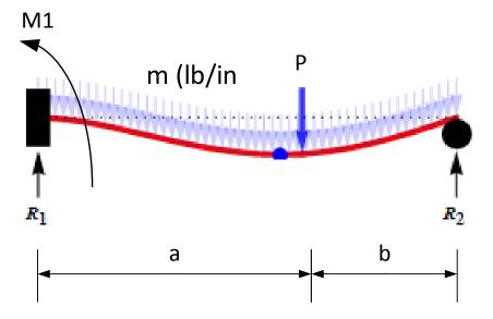
Using the following values:  $a=0.625L, b=0.375L, E=30\times 10^6$  psi (steel),  $I=57~in^4, L=144$  in, P=1000 lb, m=200 lb/in.
