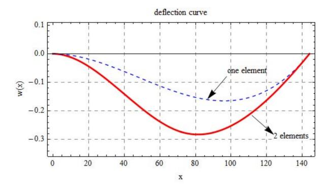
The analytical deflection for the beam in problem three above (fixed on the left and simply supported at the right end) when there is uniformly loaded with w lbs per unit length is given by
