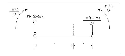
Equivalent load for the uniform distributed loading is
