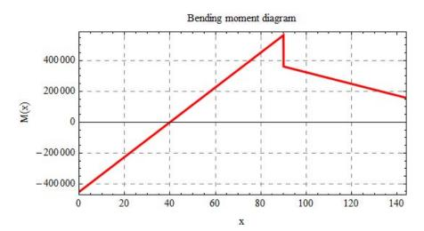
The reason for this is because the solution v(x) obtained using the finite elements method is a third degree polynomial and after differentiating twice to obtain the bending moment  $(M(x) = -EI\frac{d^2v}{dx^2})$  the result becomes a linear function in x while in the analytical solution case, when the load is distributed, the solution v(x) is a fourth degree polynomial. Hence the bending moment will be quadratic function in x in the analytical case.
