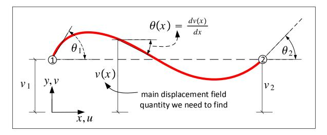
In the direct method of finding the stiffness matrix, the forces at the ends of the beam are found directly by the use of beam theory. In beam theory the signs are different from what is given in the first diagram above. Therefore, the moment and shear forces obtained using beam theory ( $M_B$  and  $V_B$  in the diagram below) will have different signs when compared to
