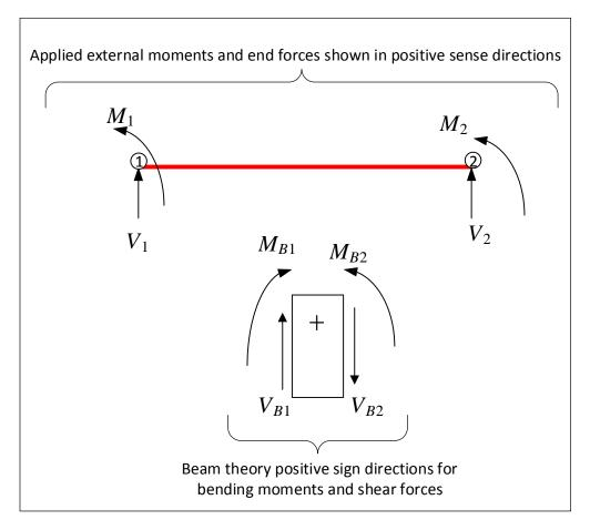
The goal now is to obtain expressions for external loads  $M_i$  and  $R_i$  in the above diagram as function of the displacements at the nodes  $\{d\} = \{v_1, \theta_1, v_2, \theta_2\}^T$ .
