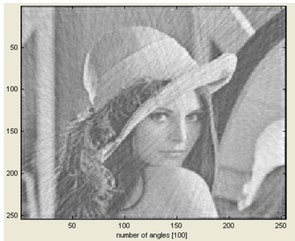
Reconstruction, 100 projections, Filtered backprojection (RAM-LAK filter)
